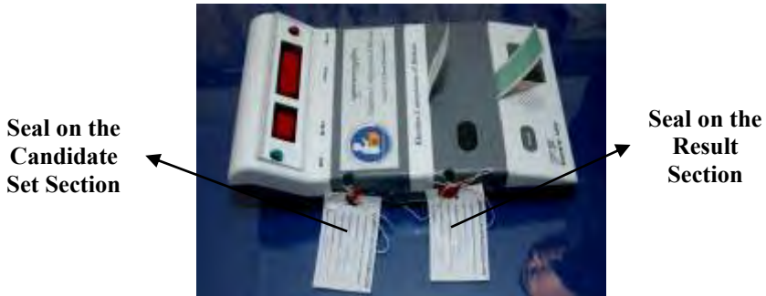
Fig. 7.5: Sealed Control Units
